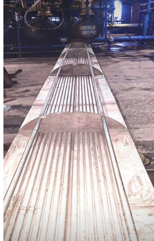
New tube bundle with Alleima 316L Tubes
